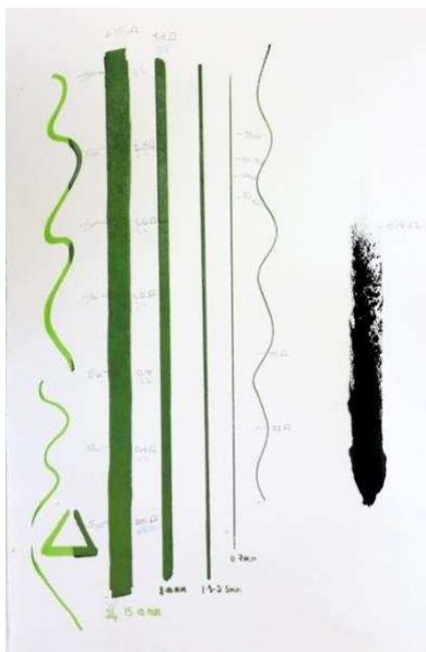
Figure 5. Screenprinted conductive ink evaluation of resistance readings
