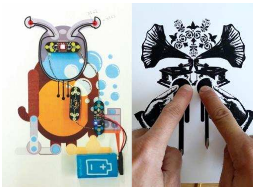
Figure 3. (Left) Silver ink and conductive thread can power a series of LEDs. (Right) Screenprinted carbon Ink on paper reacts well when activated by touch
